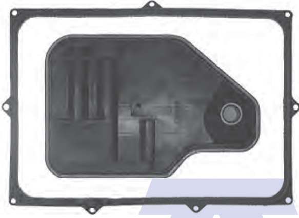
M72, 85, 91, 93, 95, 97LE Pan Gasket BTR74.GAS01 Filter BTR85.FIL01 Neck 25mm High
