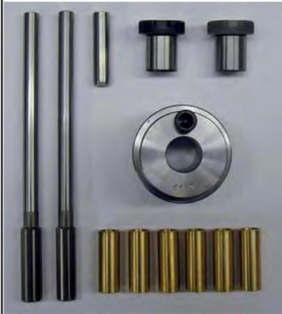
**SF-99 Servo Bore Repair System
