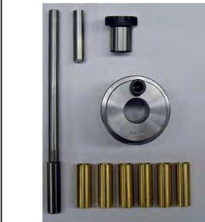
**SF-99 Servo Bore Repair System
