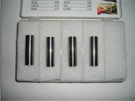
In order to get the best possible seal from the bushings we use, we machine them as close to the size of the pins as possible. However, in order for the bushing to seal and stay in place, it is necessary for the bushing to crush during installation. This "crush" effectively shrinks the bushing's inner diameter. These pins allow you to quickly and easily re-size the bushing to it's correct (something old servo pins don't always do) inner dimension.
