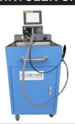
Test the transmission with fluid under pressure, the Hydraulic Tester simulates operating conditions in the unit and finds problems instantly. The Hydraulic Tester finds hidden defects in soft parts or can alert you to hard parts that have grown out of tolerance. A simple hook up to a unit test plate and the reading of a single gauge allows you to test a transmission in or out of the vehicle
