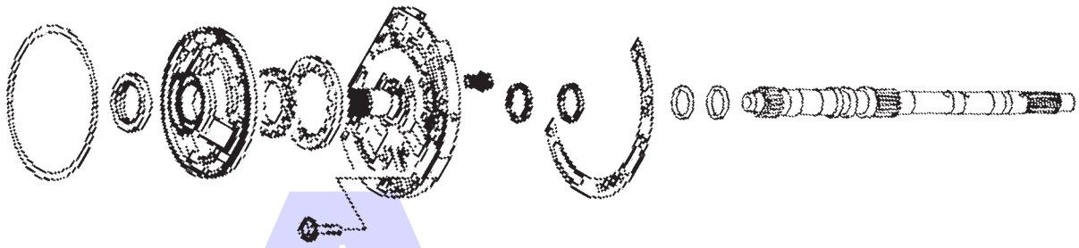
Pump & Input Shaft
